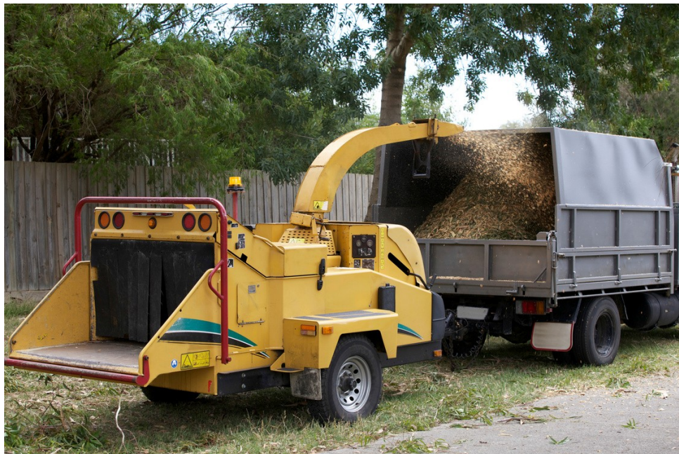
Figure 9. Usage of wood chipper to dispose of large leftover wood
